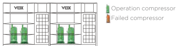
Intelligent load-bearing between units during normal operation
